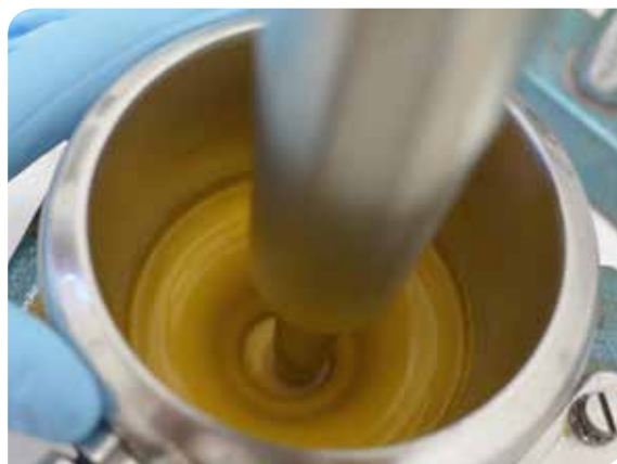
Fig 4. Iron oxide yellow colorant preparation with Phospholan PE169
