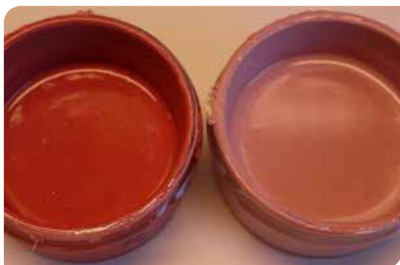
Fig 3. Alkyd paint with colorant. Left can: addition of 1 wt% Phospholan PE169 added in base paint
