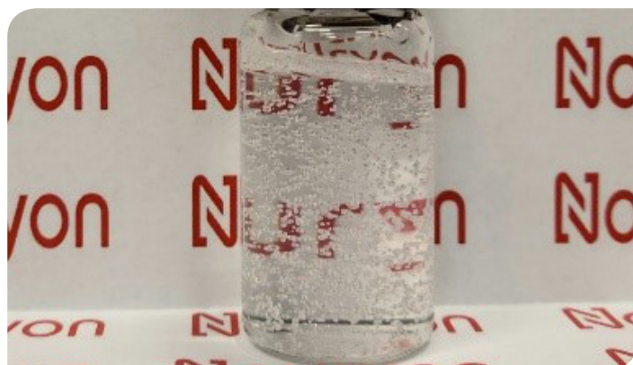
Figure 2. Clear hand sanitizer gel formulated with Structure 2020 – 16.6% Structure 2020 (5% total active) in 70% ethanol
